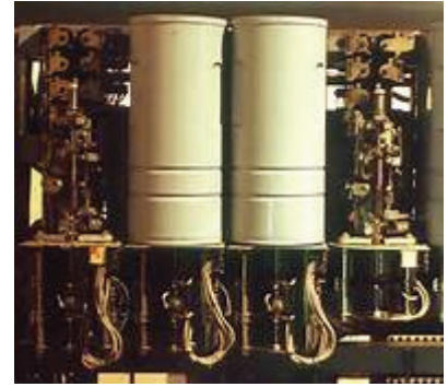
Strowger SXS Line Finder. The two center units are covered with the "coffee cans" and the two exterior units exposed.
